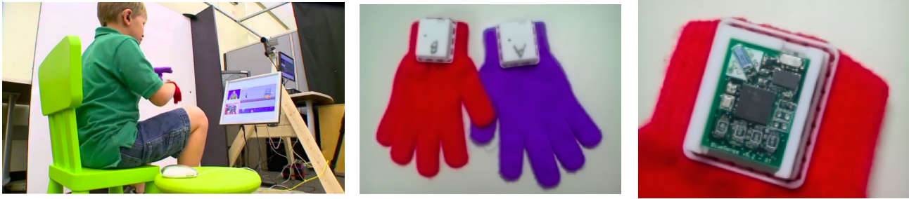
Figure 4: Originally, CopyCat used specially-designed kiosk (left) and custom sensor gloves (center) with embedded accelerometers (right) to achieve sufficient recognition accuracy for gameplay.
